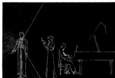
3. 120° pick-up angle lessens need for tilting.
